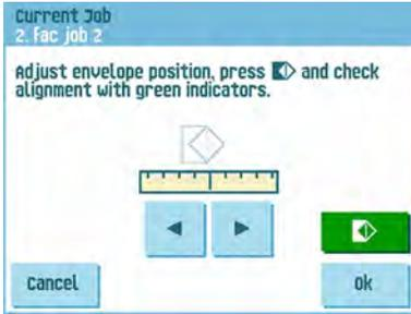
4. Press the **[OK]** button to accept the new alignment.
