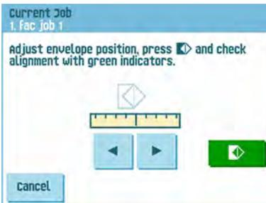
2. Use the arrows beneath the ruler to adjust the envelope position.
