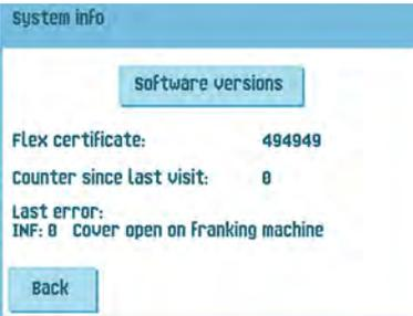
2. Press the **[Software versions]** button to view information on the version of the installed software.
