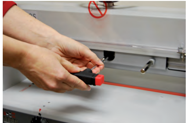
Blade change safety tool in place
