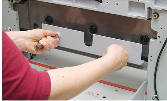
7. With the blade change safety tool in place, use the T-wrench to remove the center screw.
