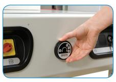
Electronic Back Gauge Adjustment Fine-tune control for precision cutting
