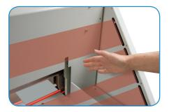
Infrared Light Beam Safety Curtain Immediately stops operation if the light plane is interrupted
