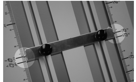
Fig. 2c Setting fold stop
