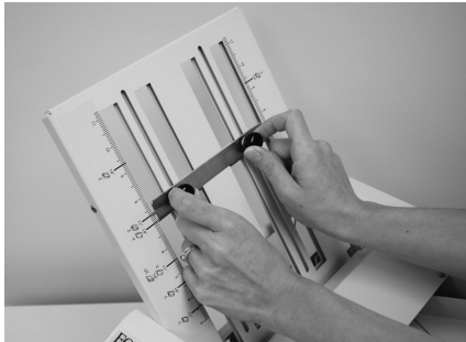
Fig. 2a Adjusting upper fold plate
