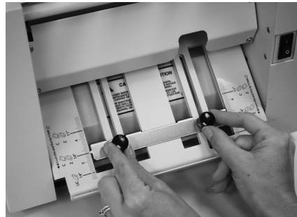
Fig. 2b Adjusting lower fold plate
