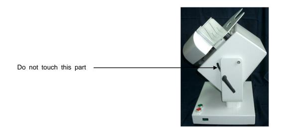
· In general, for thick paper, the tilt angle is adjusted vertically and for thin paper, it is adjusted horizontally.
