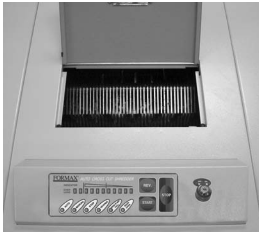
Control Panel and Cutting Block Access Door
