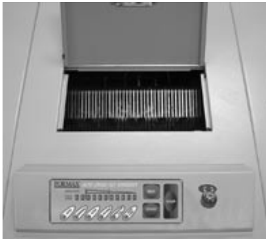
Control Panel and Cutting Block Access Door
