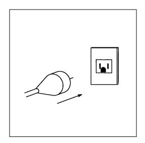
Insert the power cord into the inlet. When the power switch is on, the stoppers of Table 1 and 2 move to the home position.
