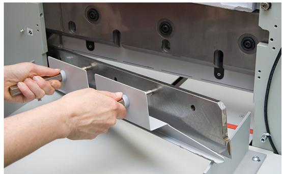
9. Carefully remove the old blade from the blade change safety tool. Set it on a flat surface and unscrew the handles. Cap the old blade with a protective pad to prevent injury.
