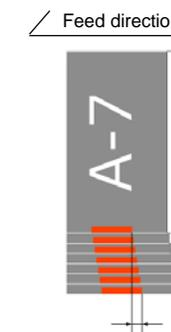
If the images on the cards are shifting as shown in the drawing B, the length of gutters should be decreased.
