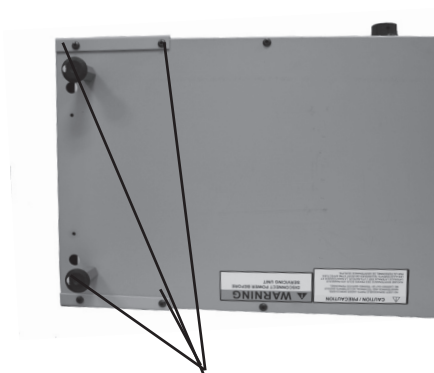
Fig 1a Mount the side guides using these screws.
