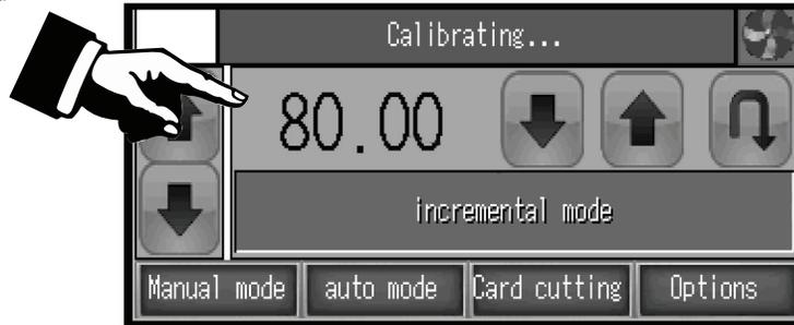
To move the back gauge in increments by the same dimension multiple times (forward or back), input this dimension by pressing it on the screen and using the on-screen keyboard.
