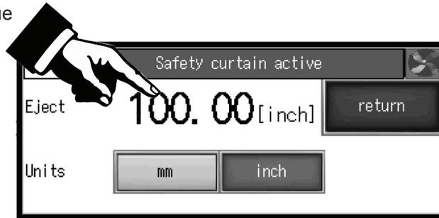
Eject can be set in inches or mm. It is the value by which the paper stack moves forward at the end of a cycle. After each cycle, the back gauge returns to the previous position. Enter the value, then press **RETURN**.
