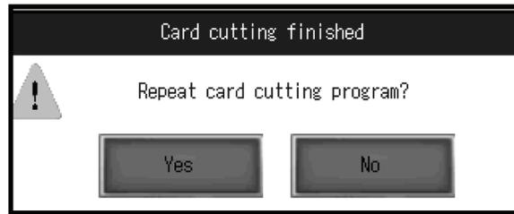
Pressing **YES** moves the back gauge automatically into the first dimension to repeat the same program. Pressing **NO** exits the program.
