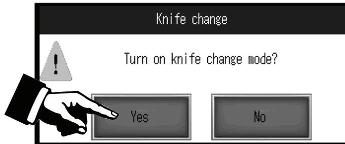
Press **YES** and make a cut by pressing the two cut buttons on the front of the cutter. This will put the knife in the lowered position, ready to be changed. Change the knife according to instructions in Operator/Maintenance Manual.
