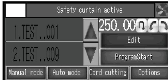
When selecting a saved program, it's possible to check the steps and dimensions written in the program (using the up/down arrows), and if the step has active functions (eject, paper rotation, etc.).
