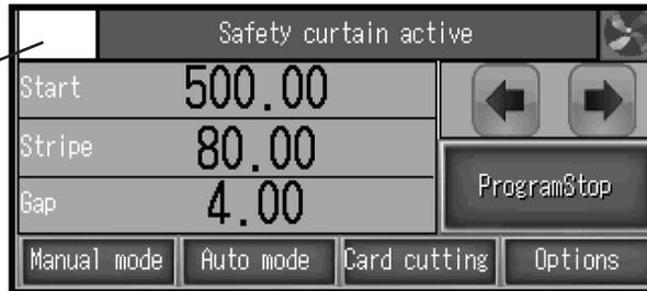
The back gauge moves into the starting position for the first dimension and after each cut, it moves automatically to the next step.
