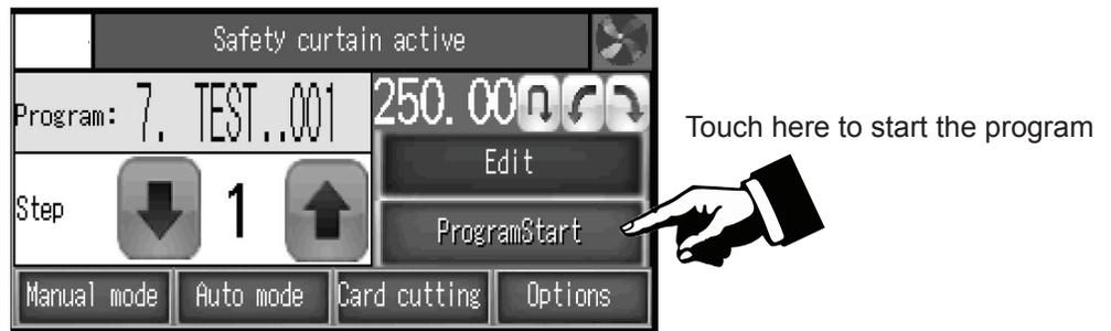
After pressing Program Start, the back gauge moves to the dimension saved in step 1 and a new screen appears:
