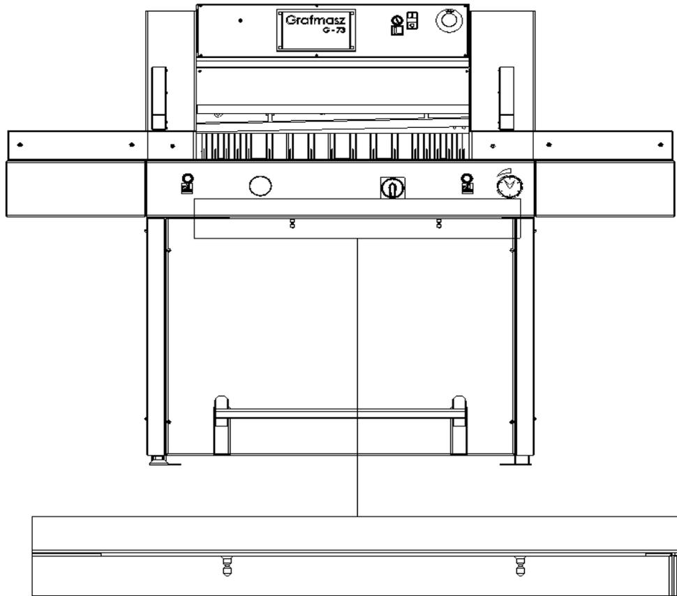
Drawing 33. False clamp location (before fixing on the clamping beam)
