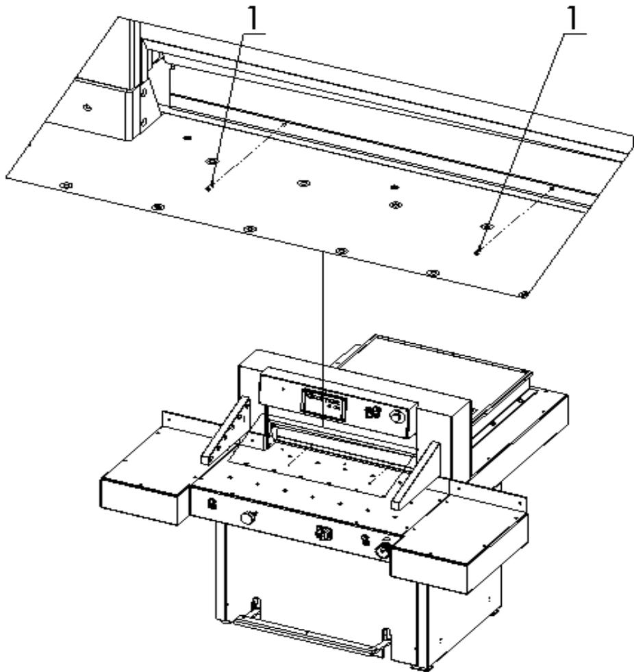
Drawing 35. Location of the screws, which block the false clamp
