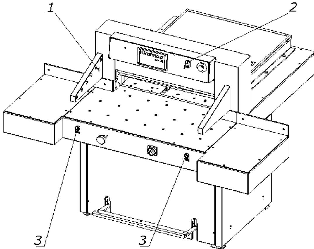
Drawing 13. Operation and signalization during cutting
