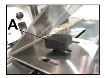
**3.** Install the Rear Media Guide using the thumbscrew [**B**] and washer provided. The washer goes between the screw and the Rear Media Guide Support.
