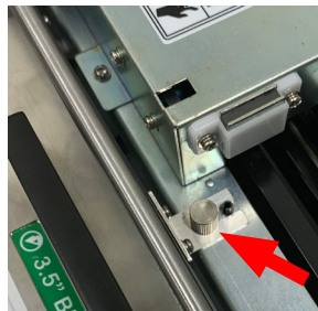
5. Remove thumb screw and remove blade cassette
