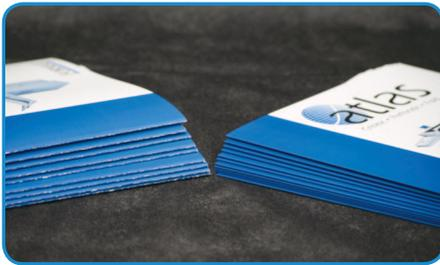
*Uncreased folded digital prints (left) are cracked and give the appearance of poor quality. Creased prints (right) have no cracking and look polished and professional.*
